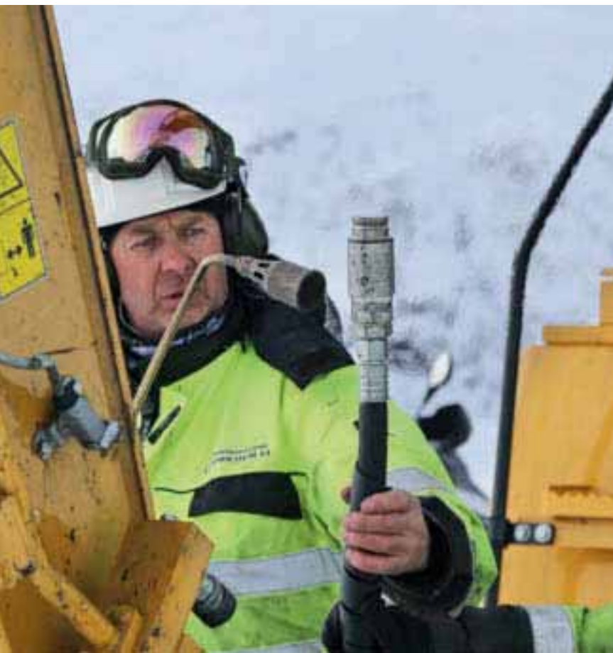
FRYSER: En hurtigkobling krangler i kulda.
